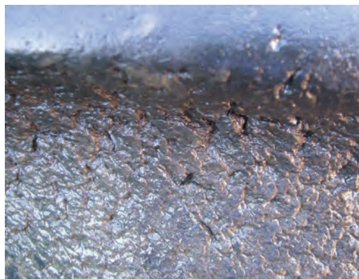
These photos show how soybean and corn stubble can pit the rubber of farm tractor tires.
