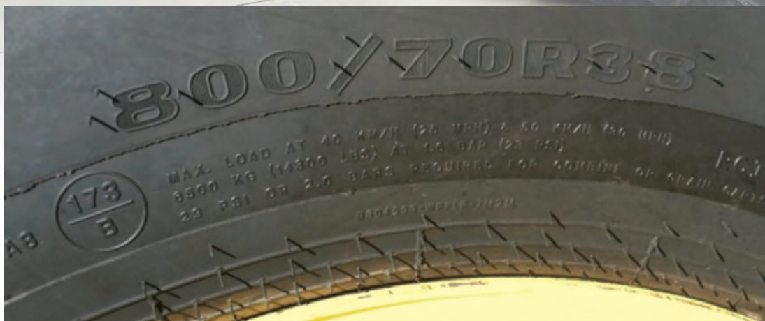
A radial agricultural tractor tire that is 800 millimeters wide, has an aspect ratio of 70, and fits on a 38-inch rim.
