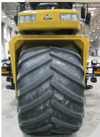
Tractors and self-propelled equipment have drive wheels that have heavy-duty treads (called cleats or lugs). Cleats grab the ground and help move the equipment forward through loose substrate.
