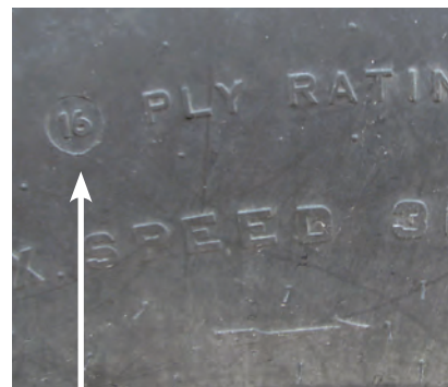
A tire with a 16-ply rating is equal to a tire with an H load rating.
