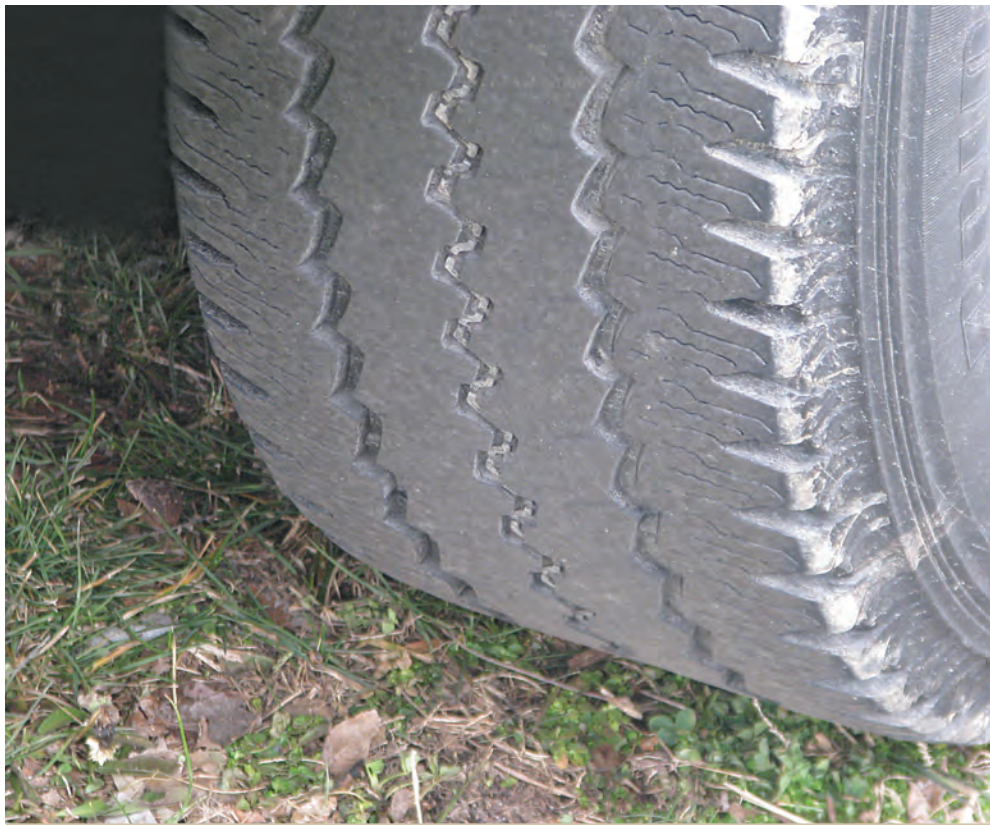
An overinflated tire wears more in the center of the tread.
