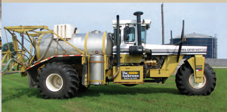
Tractors and self-propelled equipment have drive wheels that have heavy-duty treads (called cleats or lugs). Cleats grab the ground and help move the equipment forward through loose substrate.
