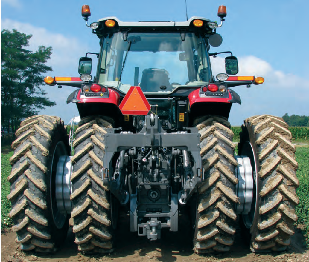
Tractors and self-propelled equipment have drive wheels that have heavy-duty treads (called cleats or lugs). Cleats grab the ground and help move the equipment forward through loose substrate.
