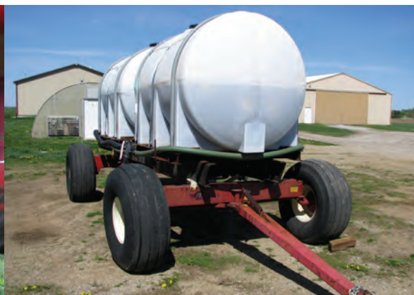
Many implement tires have unaggressive treads like trailer tires. That's because implements will be pulled, so their tires are constructed to carry weight at slow speeds without compacting soil. They are not designed for maneuverability or comfort.
