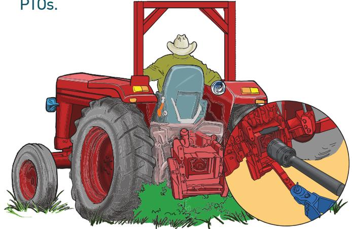
Turn off power when connecting, disconnecting or servicing a machine.
