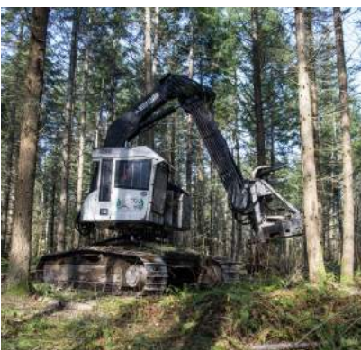
Tracked equipment has less soil impact than vehicles with tires. Photos: Matt Freeman-Gleason
