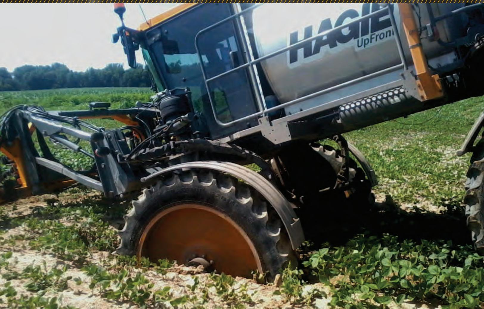
It takes more pulling strength to move something mired in the ground than it takes to pull the same object over the road. When you tow something on the road all you have to do is get the weight of the towed vehicle moving forward.
