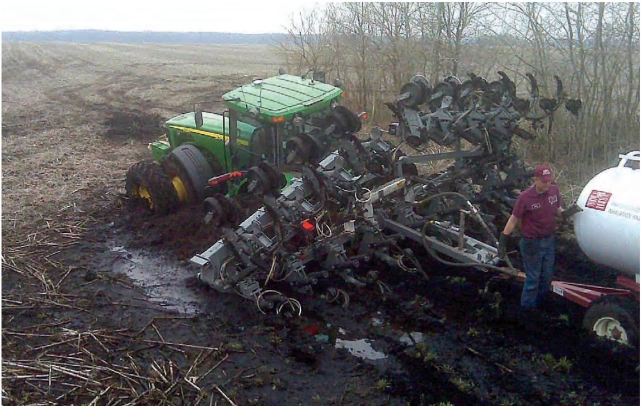
*You need to be especially careful in a situation like this. Inspect all hoses and fittings after the tractor and wagon are pulled out to make sure no anhydrous has leaked. And before you try to make any extraction consider whether the wagon should be pulled out backward, and the anhydrous ammonia tank valves have been shut off.*
