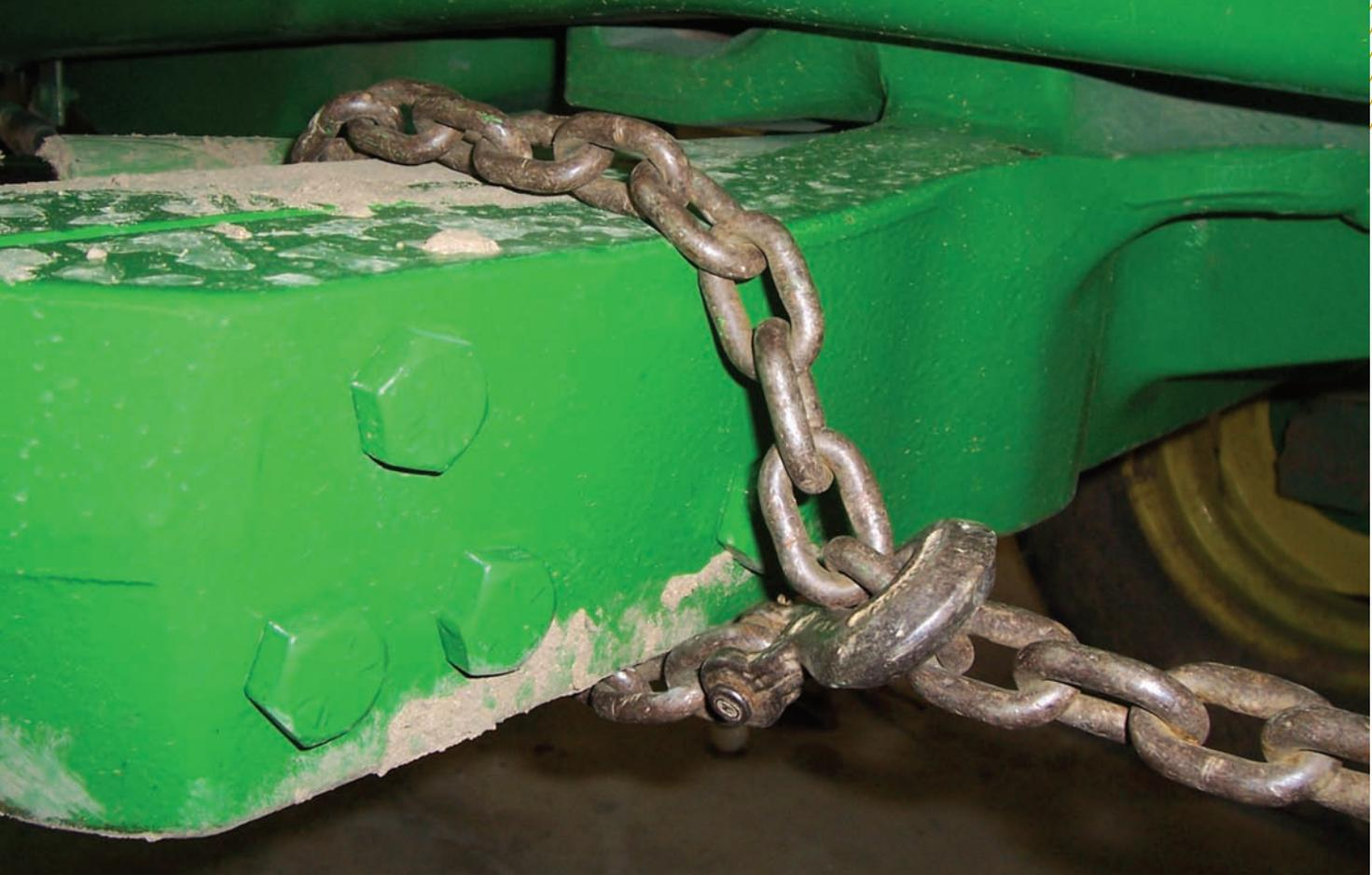
*Grab hooks are designed to slide over the full link. Don't hook the tip of the grab hook into the opening of the link pulling on the tip of the hook. Pulling on the tip of the hook compromises the design capabilities of the grab hook. The full strength of the grab hook can only be achieved by sliding it fully over both sides of the link.*
