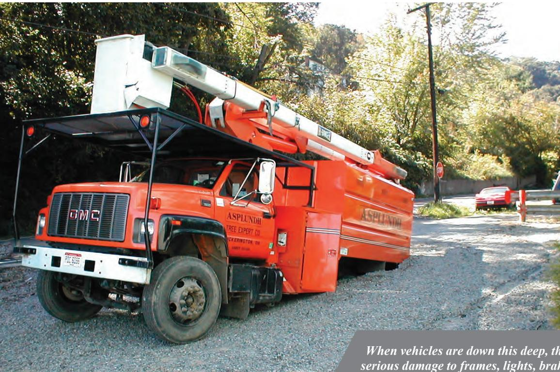
*When vehicles are down this deep, there could be serious damage to frames, lights, brake lines, tires, hitches, fuel tanks, and exhaust systems. Don't put defective equipment back on the road. Take a few minutes to inspect all equipment after any extraction.*
