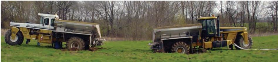
The two attachments points are to the towing vehicle and the stuck vehicle. It is not a good idea to hook multiple chains, straps, or ropes together. For instance, if you attached two, 30-foot ropes together, the real issue will be the clevis that connects the two ropes in the middle. The amount of force you generate could snap one of the ropes. If you need more length than what you have, call a wrecker service.
