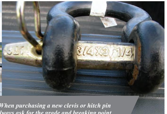
*When purchasing a new clevis or hitch pin always ask for the grade and breaking point. Never assume it is strong enough to do every job based on weight and appearance just because it is new.*
