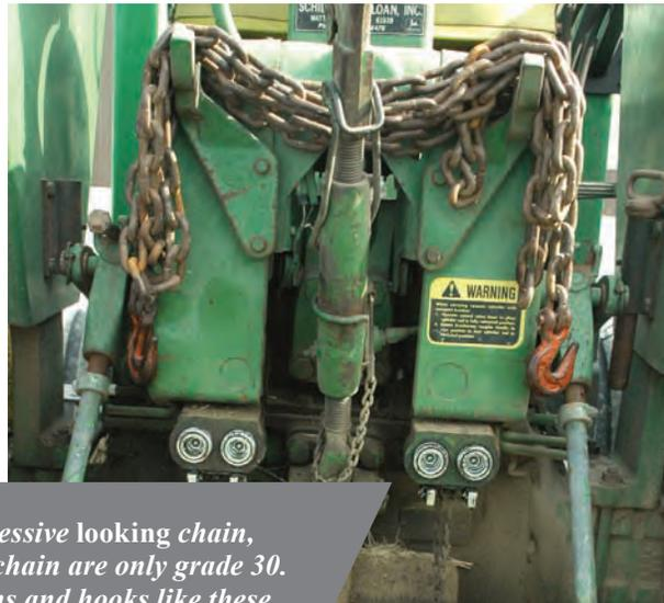
*This is an impressive looking chain, but the hook and chain are only grade 30. Low-grade chains and hooks like these will meet their match and break.*
