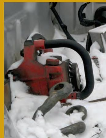
*It defies logic and common sense to leave any of the recovery devices in the back of a truck bed. Doing so will cause the metal to rust and the nylon straps to be degraded by sunlight.*
