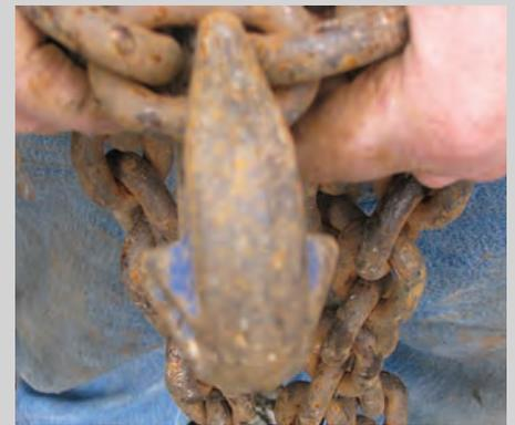
*Never use a chain if its hooks have been altered in any way or if the hooks' ratings are not equal to or greater than the chain's rating. Certain hooks have wings or ears on them to keep the chain from pinching too tight around the hook. It allows the force to be distributed on all links instead of just one.*
