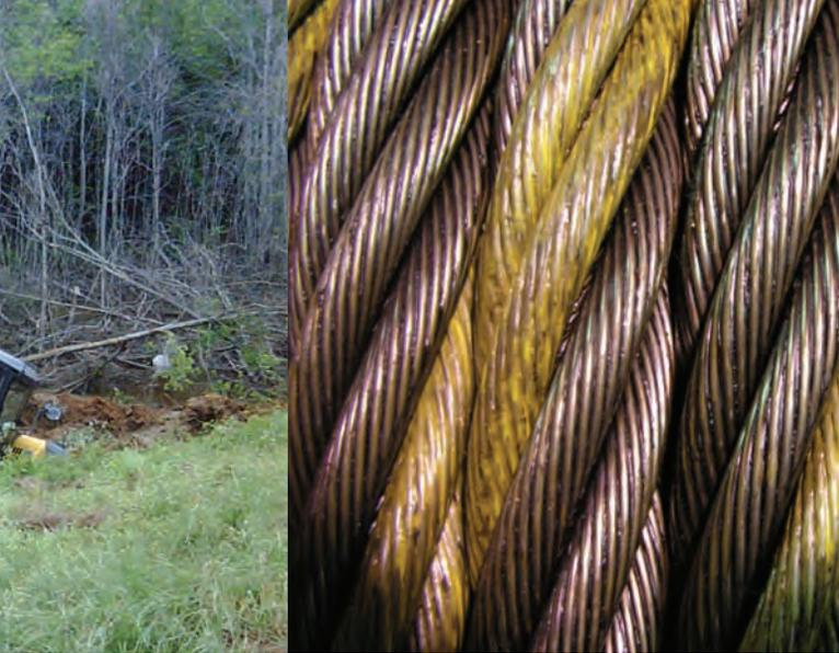
You also have to pay attention to how many of the wires are cut — if enough get cut, the integrity of the cable will be compromised. Each cut or broken strand reduces the cable’s overall strength.
