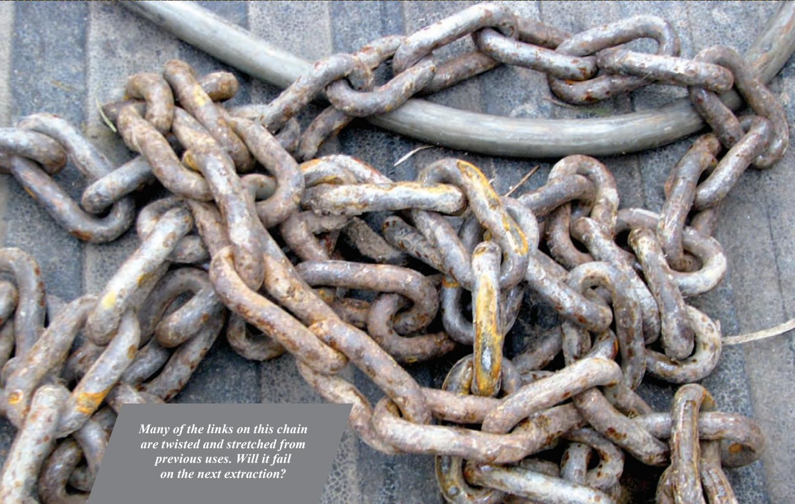
*Many of the links on this chain are twisted and stretched from previous uses. Will it fail on the next extraction?*
