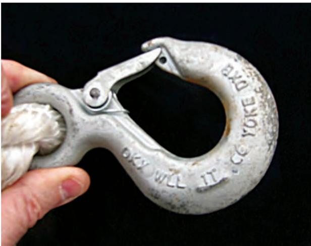
*This tow rope has a hook that is rated at 1 ton. But this equipment is not rated for anything more than towing a lightweight vehicle on the roadway. In addition, the latch cannot take any weight.*
