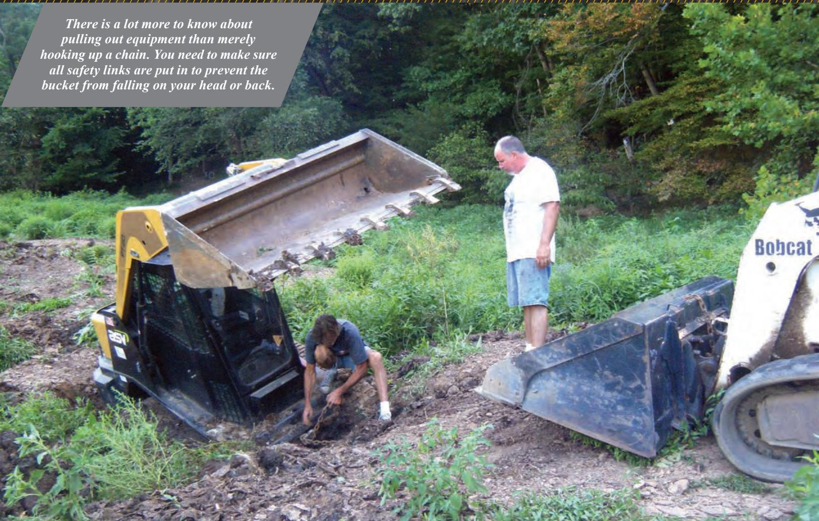
Before you try to extract any stuck vehicle with a cable, rope, or chain, consider the 28 tips described below. Remember, your goal is to have the pulling force exceed the immovable force — only then will the truck or stuck equipment move forward. If there is not enough force pulling forward, then whatever is stuck will not move.
