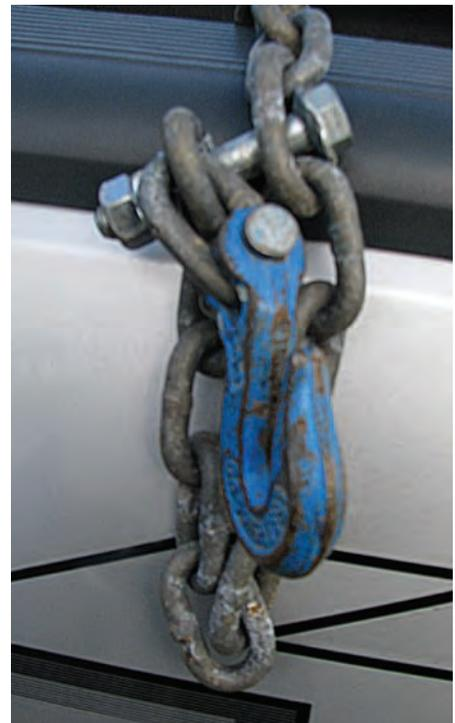
*Never make a loop at the end of a chain and attach it with a bolt. This compromises the strength of the chain. The chain's strength is no longer the weakest point or limiting factor. Now, all of the force will be placed on a loosely tightened nut. Bolts are made to work when they are tightened down for whatever they are holding. Use the chain and the hooks as they are intended to be used.*
