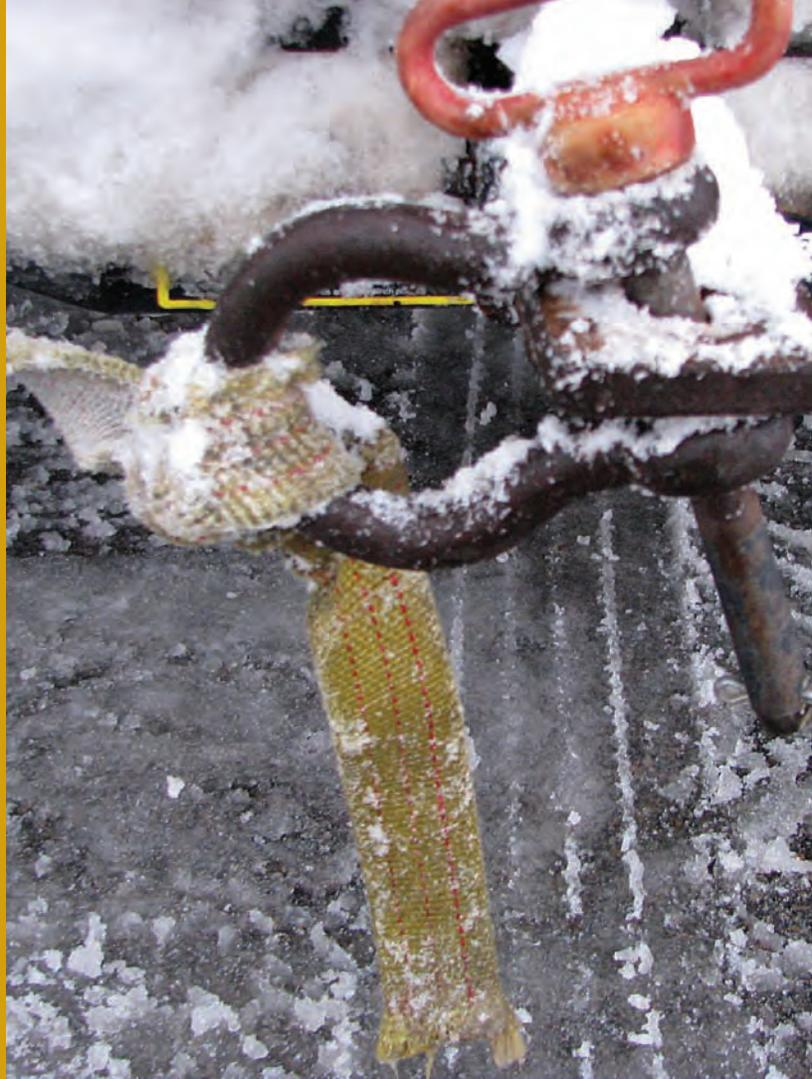
*After this strap was torn, the operator tied a knot around the clevis and continued to pull equipment. The question is whether the knot, hitch, and pin will hold when pulling equipment stuck in snow or in mud. Past experience says it may, but the reality is it won't.*
