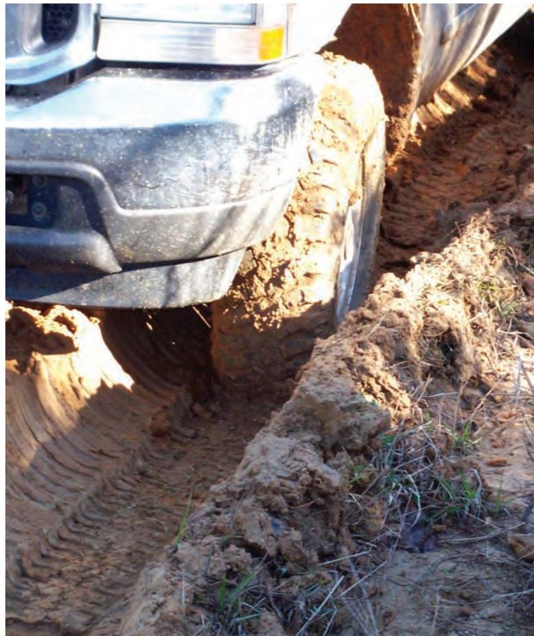
Ideally, you want to position the towing vehicle on higher ground. This will give you a mechanical advantage to overcome and negate the forces that hold the stuck equipment in the mud. It is easier on the towing vehicle if it can pull the stuck vehicle's wheels up and out of the hole and onto solid ground. If the towing vehicle is pulling forward or downward, it is forcing the stuck equipment into the immovable ground.
