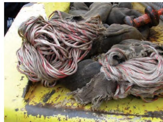
It doesn't matter whether it's a rope, strap, cable, chain, or hook. You should only store a device if it is in good operating condition. If your strap is cut, its strength capacity is less than its rated capacity. If your recovery chain has stressed links from the recent pull, then that's where it will break the next time it is put under stress. If your rope is frayed because it was laying on a sharp edge, you have compromised its ability to carry the load it was rated for when new.
