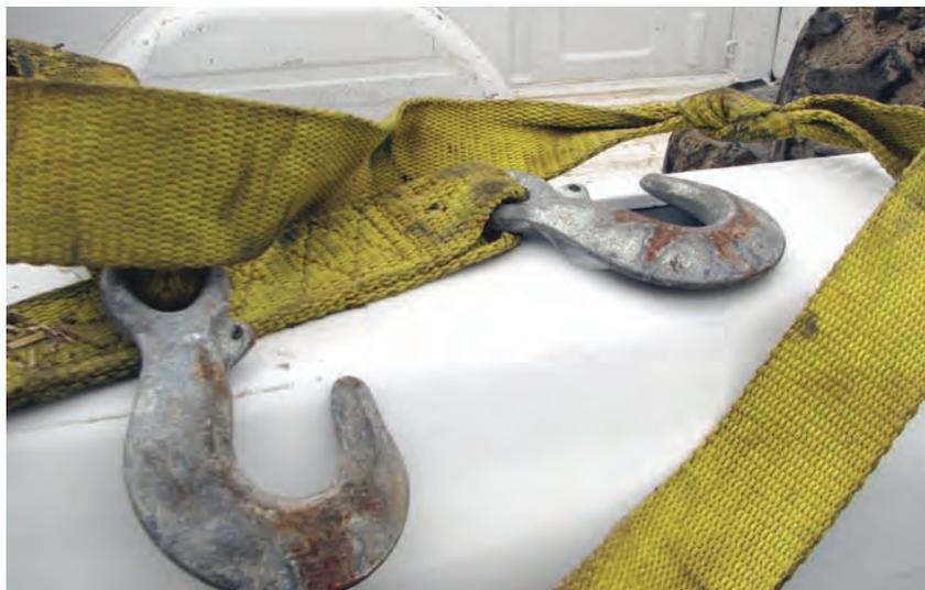
***Knots significantly reduce the strength of any strap or tow rope. Straps are designed to be used flat. Knots reduce the strength of the web when it is bunched together and twisted into a tight knot. All of the tension is placed on less area.***
