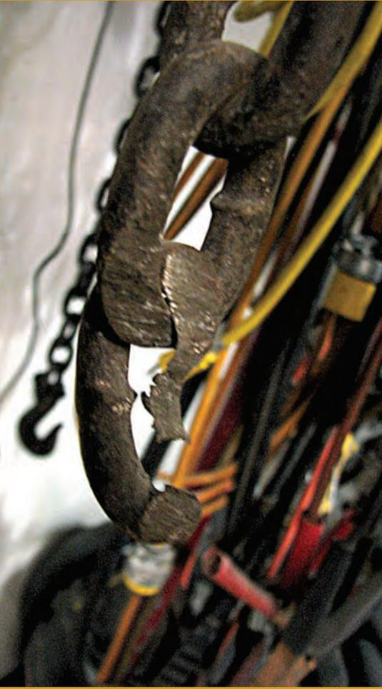
*Chains are important for any farm or business. However, unless the chains have been inspected for faulty links, they will have limited use for extracting stuck equipment. Notice one of the links that was dragged on the ground and one with a broken link. Never put damaged chains back in service.*
