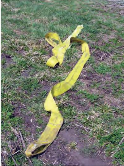
There are many instances where metal at one end or the other can be attached to a tractor or truck through a hitch. When attaching a rope or strap to a tractor, the preferred point of attachment is the drawbar because it is designed to carry heavy loads. Make sure the hitch pin and safety pin are strong enough to prevent the clevis from separating under pressure.
