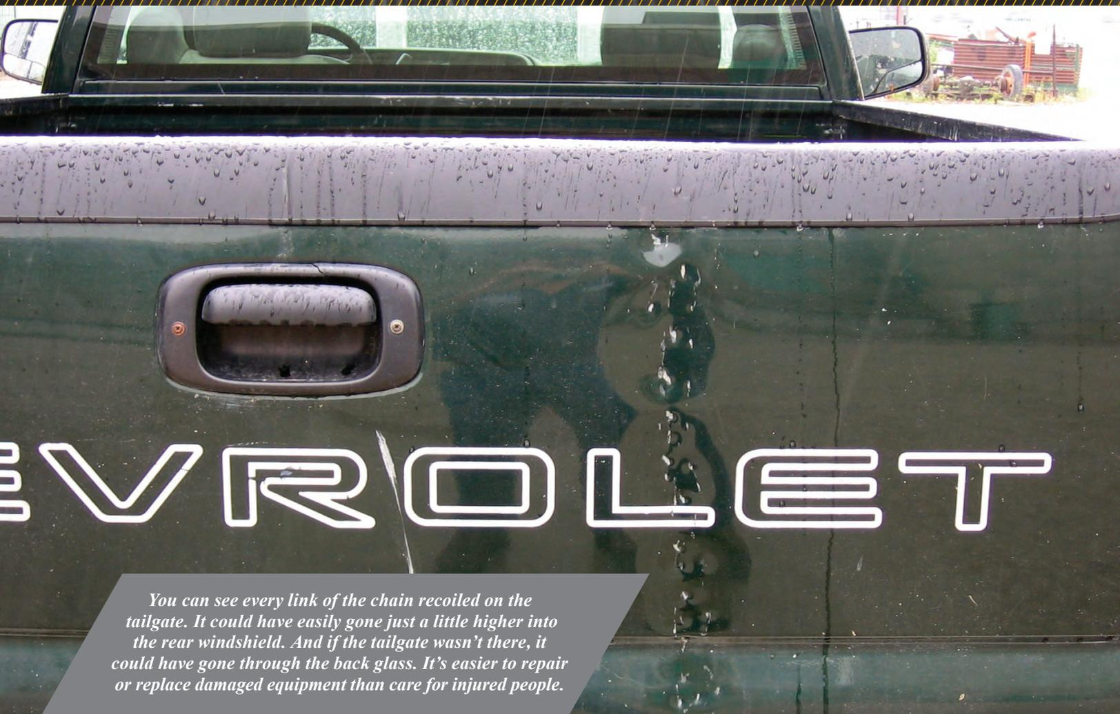
*You can see every link of the chain recoiled on the tailgate. It could have easily gone just a little higher into the rear windshield. And if the tailgate wasn't there, it could have gone through the back glass. It's easier to repair or replace damaged equipment than care for injured people.*
