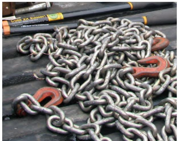
*Never assume that a strong chain is enough. Always determine the strength of the hooks. The breaking point is the lowest number of the two.*
