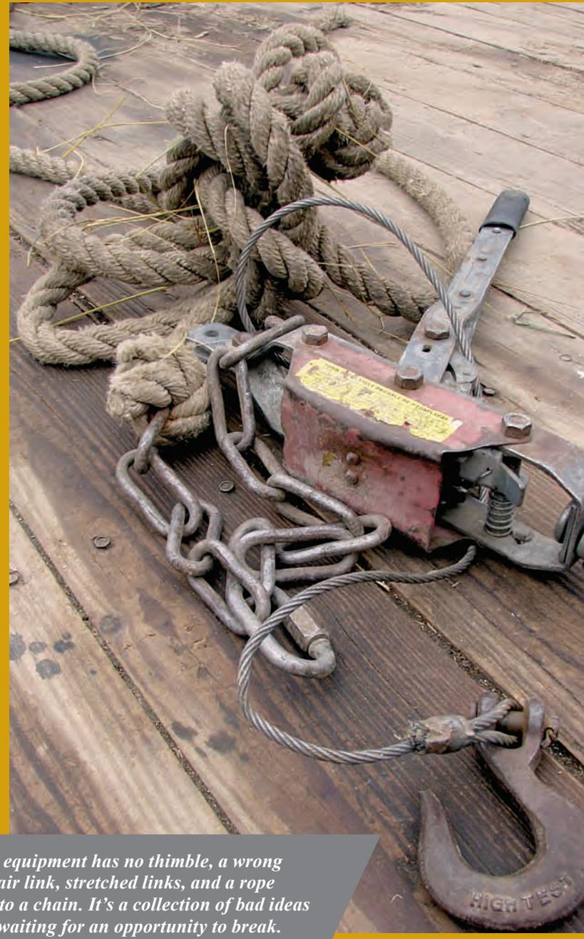
*This equipment has no thimble, a wrong repair link, stretched links, and a rope knotted to a chain. It’s a collection of bad ideas just waiting for an opportunity to break. Use the proper equipment rated for the job.*
