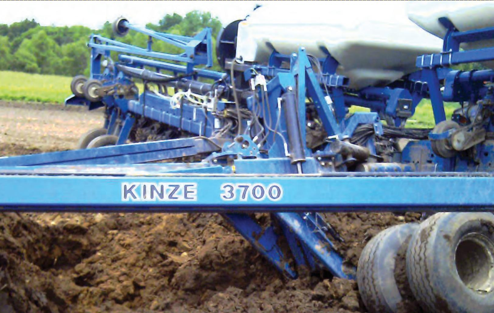
One of the most obvious (but overlooked) things to do is to inspect the equipment that you pull out after the extraction. The deeper the equipment was mired in mud, the more important the inspection is.
