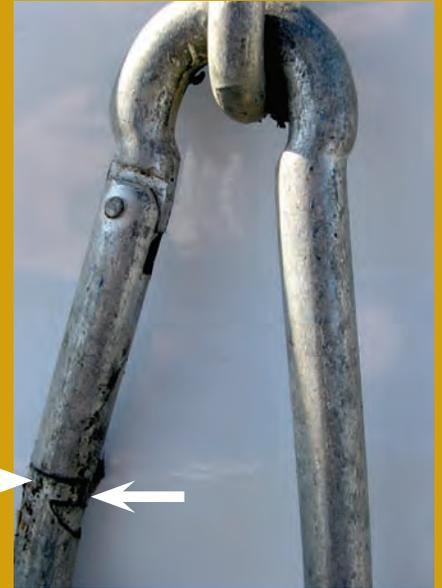
*While commonly used on chains, these connectors cannot stand the stress they will encounter during vehicle or equipment extraction. Notice how little metal there is on the post. This greatly weakens the connector.*
