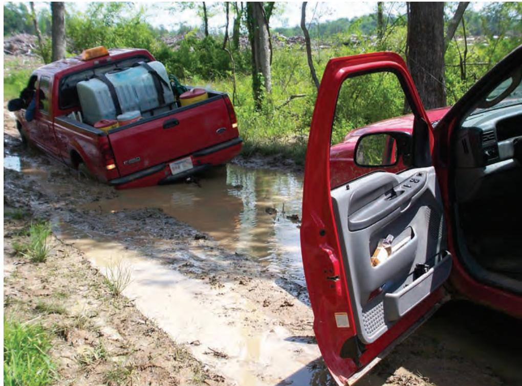
***What are the odds that this truck can be pulled out of the mud without jerking on the chain? Probably slim to none. But jerking on the chain increases the probability that something will give way, especially when the chain is undersized or in poor condition.***
